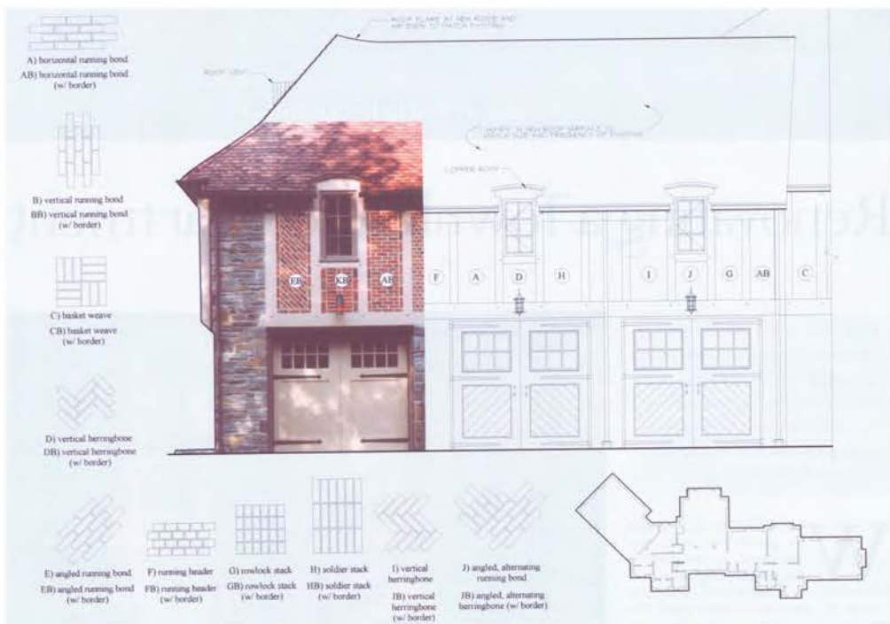
Above: The garage elevation reveals the individual brick nogging panels between half timbers.
